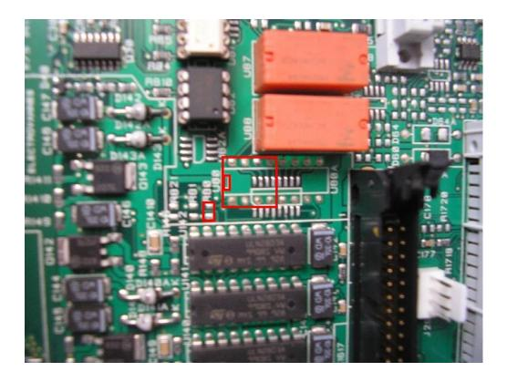
3. You have to clear the marked holes of the U80, and solder the IC socket (2x4pins). After that you have to solder the R80 resistor. For your convenience you can follow the picture, and you can use the equivalent pin from R81 which is short with R80 to make the soldering easy.
