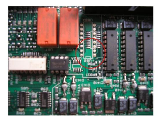
2. You will have to solder ½ of U80 circuit (TLP 621-2 opto instead of the original TLP 621-4) and the R80 resistor . This two components are responsible for the "Syncmess" signal. The original resistor value is  $R=180~\Omega$ . However sometimes you have to "calibrate" this resistor (you have to test the output – described later)
