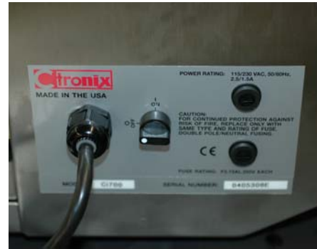
Interruptor de corriente OFF
