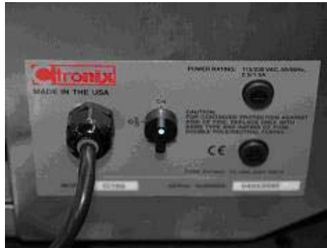
Interruptor de corriente ON
